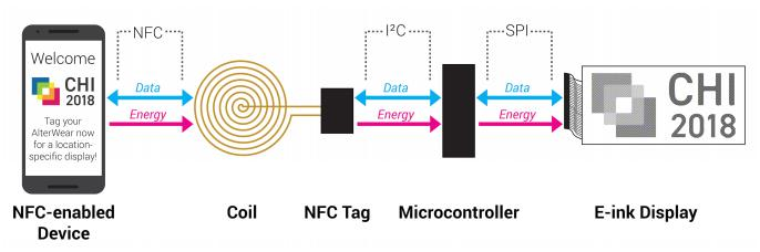
Figure 4. The AlterWear architecture includes an NFC tag, a microcontroller, and an e-ink display that are powered and updated through contact with an NFC-enabled device. When the device comes into contact with AlterWear, energy and data are transferred via NFC. The NFC tag then powers and transfers data via I2C to the connected microcontroller. Finally, the microcontroller powers and communicates with the e-ink display over SPI.
