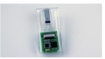
Figure 12. To demonstrate durability and longevity of AlterWear devices, we completely enclosed our fingernail prototype in resin. The prototype is durable, waterproof, and still entirely functional.
