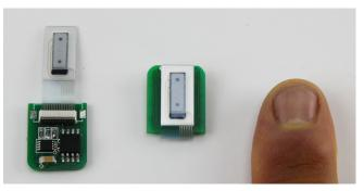
Figure 8. The fingernail AlterWear design with custom circuity and eink (Left) and folded over into a more compact fingernail form factor exposing the dynamically programmable e-ink dot pattern (Middle) next to an actual fingernail (Right).
