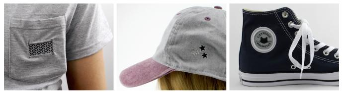
Figure 1. Three AlterWear prototypes. Note how well the technology is integrated into the garments. Left: Tee shirt pocket display (i.e. pattern). Middle: Segmented hat display (i.e. stars). Right: Discreet sneaker display (i.e. Catverse logo). AlterWear couples energy harvested from an NFC-enabled device with e-ink displays to afford dynamic interactions and expressions without the need for on-board power.
