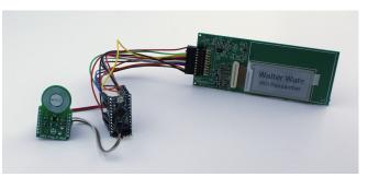
Figure 3. Our larger prototypes use an NFC Tag 2 Click breakout board, an Arduino Pro Mini microcontroller, and an e-ink display with EPD Extension Kit. While these components are relatively large and bulky, the size can be significantly reduced with custom hardware (see Figure 8).
