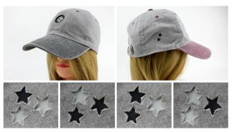
Figure 6. Baseball hat prototypes. Left: Hat prototype with AlterWear display on the front panel. Right: Hat prototype with AlterWear display on the side panel. Below: Close up of the side design. We added a simple animation when updating the display to give the appearance of sparkling or twinkling stars.
